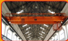
Overhead EOT Crane
